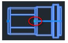
Click at this triangular grip and change the length. The shortest length is the depth of plug-in. The longest length depends at the assortment.
