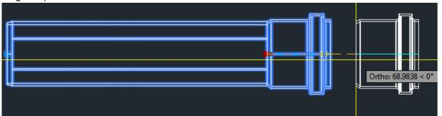
The length can be also changed in the properties of the part block.
