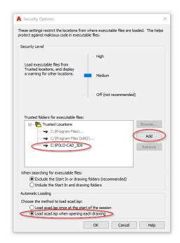
Add a Trusted folder on the right side in the window. In the new line, fill in "C:\POLO-CAD\_3De". If you change the installation path, fill in the alternative path.
