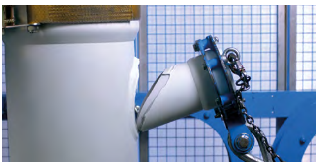
Test on POLO-ECO plus Premium DN 400/160/45° as an example
