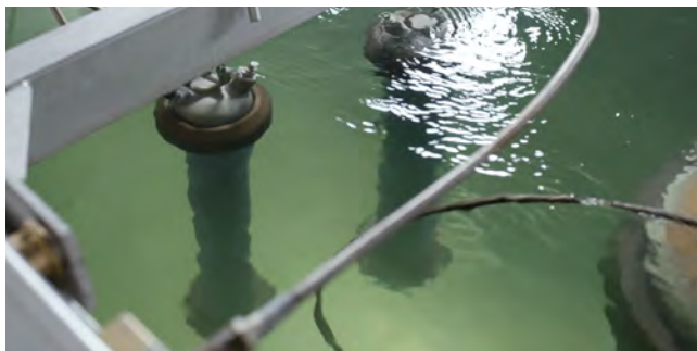
Various POLO-KAL® pipes for the internal pressure creep rupture test
