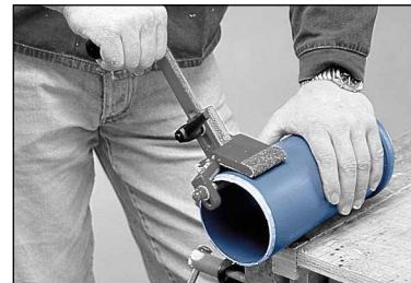
Bevelling with a bevelling tool
