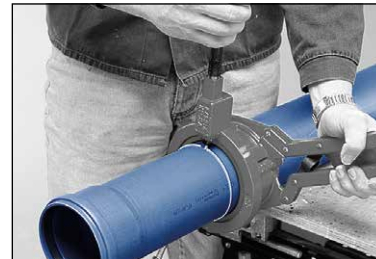
Cutting to length with a cutting and chamfering tool like this product from the company Rothenberger: ROCUT® 110/160
